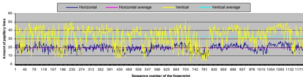
Figure 9. Numbers of papillary lines for the sensor SFM3010 [2]
