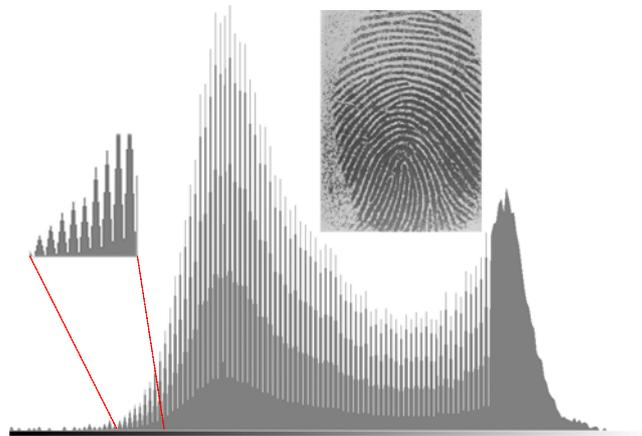
Figure 7. Histogram of the sensor SFM3050 (only a half of the x-axis is used) [2]
