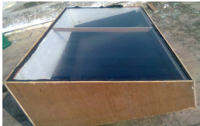
Figure.3 Solar Still Glass with Cover
