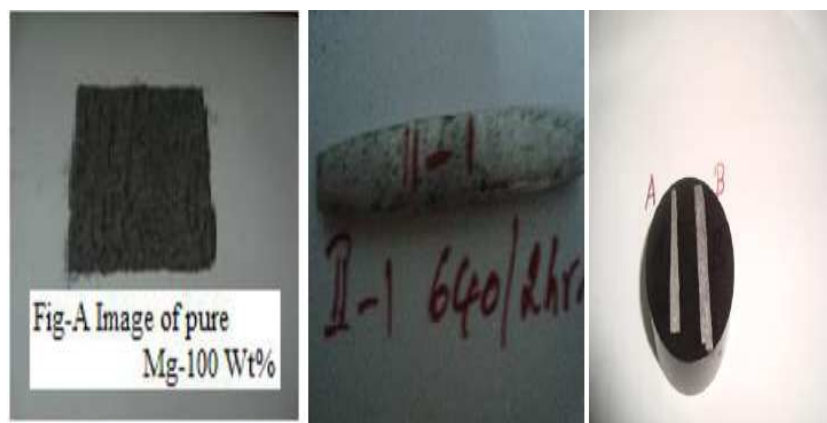
Figure 1: Images of Pure Mg different stages of Consolidation and Mounting
