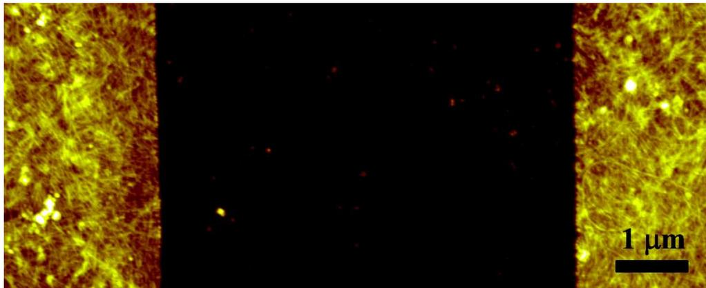
**Figure 4.** The AFM image of etched SWCNT films. The brighter areas are patterned SWCNT films, the texture of SWCNT films was shown, and the darker area is the substrate. The dots on the substrates are possibly the catalyst nanoparticles used for the growth of SWCNTs.
