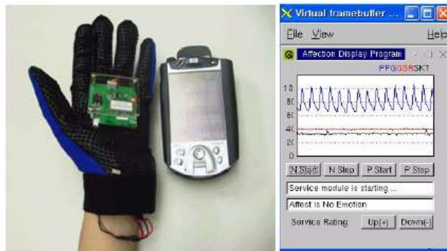
Fig. 1. The physiological signal sensing system and user interface of human status aware system
