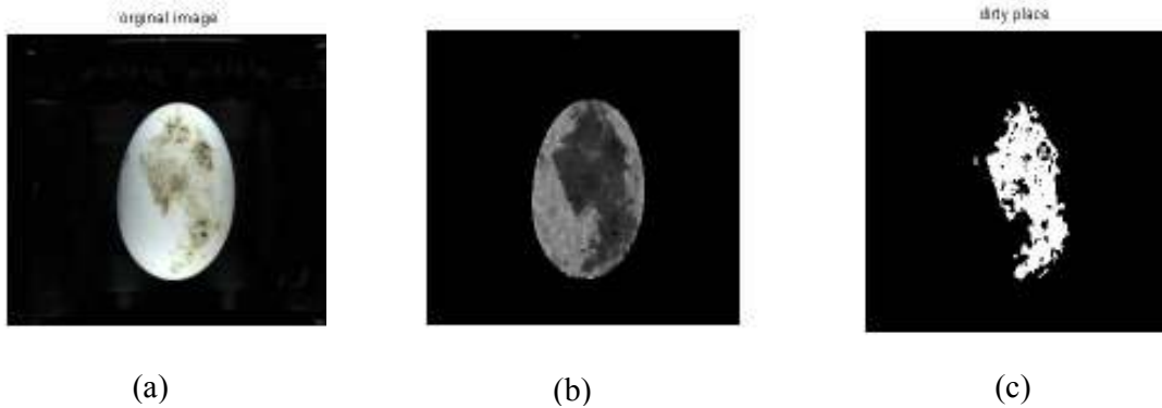
Figure 5. Successive steps (from (a) to (c)) in dirt detection on a sample with high dirt on eggshell
