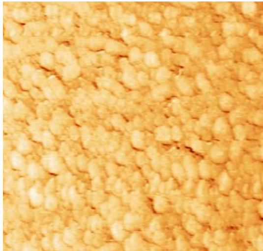
Figure 1. AFM Image of Iron Nanoparticles
