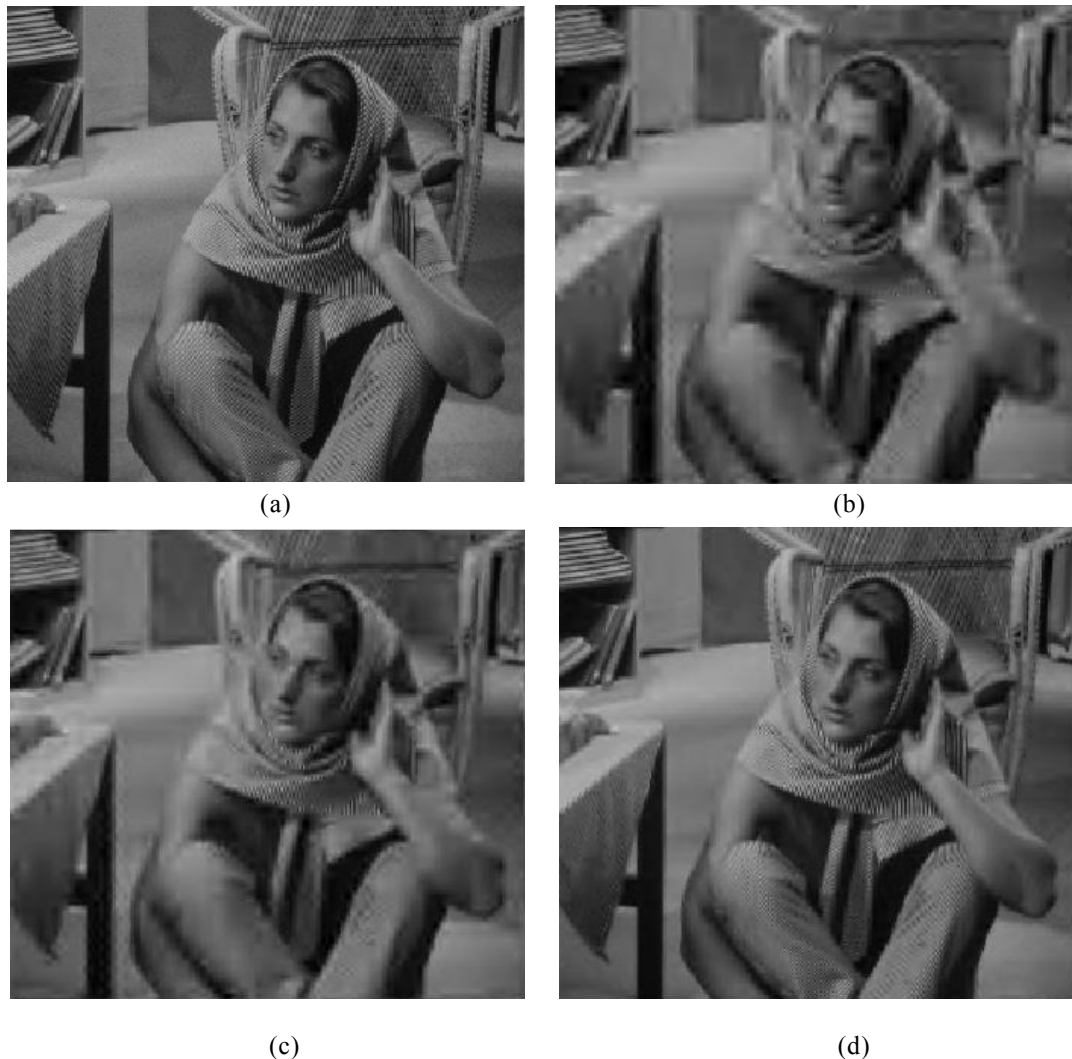
Figure. 1. (a) Original Barbara image (b) Noisy Barbara of \sigma=10 . Reconstructed images (c) DGHM (45.83dB), (d) Proposed filter (46.07 dB).
