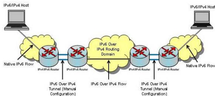
Figure 1. Manually Configured Tunnel
